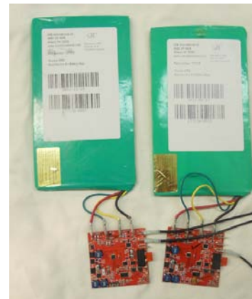
Step 2 Move middle wire from old battery (circuit board) to new battery.
