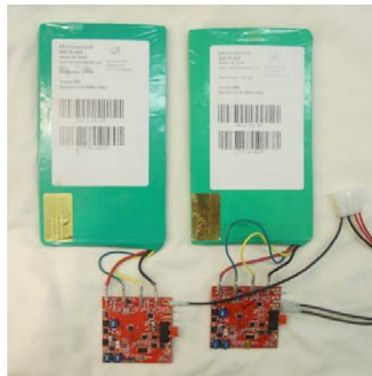
Step 1 Move top wire from old battery (circuit board) to new battery.
