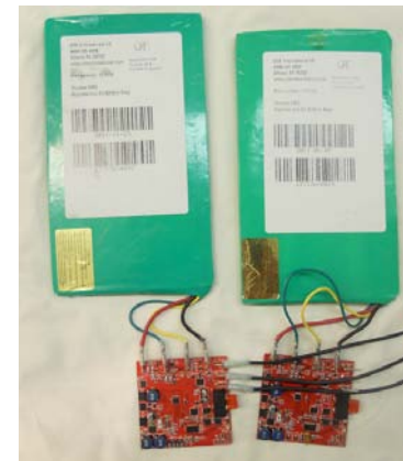
Step 3 Move bottom wire from old battery (circuit board) to new battery.
